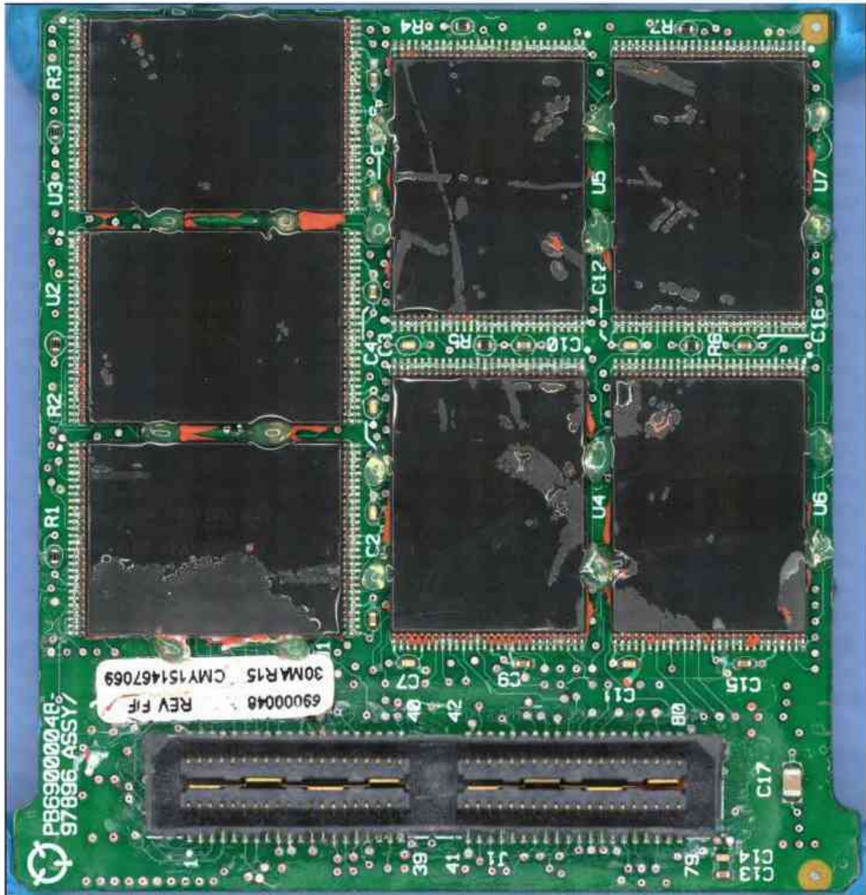
Figure 1. CVR memory module board, connector side.
